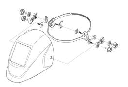
Step 1: As is shown above, pls install the adapter to the welding mask firstly.
