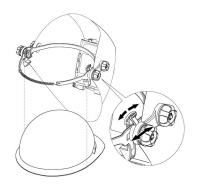
Step 2: Put the adapter on the safety hat and fasten it.
